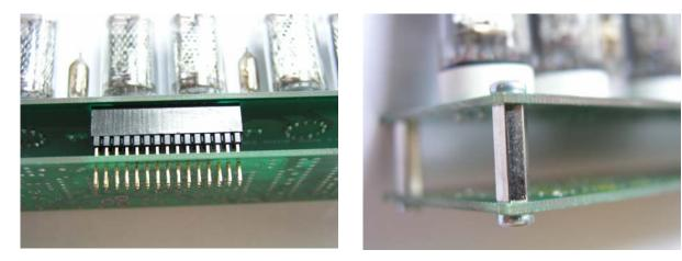
5. Solder the connector and cut unnecessary part of the pins.
