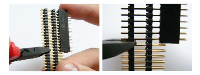
2. Cut or mill the plastic holder from the pins on the both sides.
